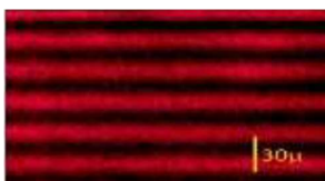
Figure 1. Optically recorded grating on NC.
