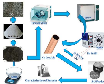
Figure 1. Experimental setup of aluminothermic reduction.
