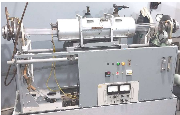
Figure 1. Experimental apparatus for producing typical layers of graphite on copper foil.
