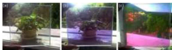
Figure 1. Temperature-dependent color change of CLC-based smart window at variable ambient temperatures.
