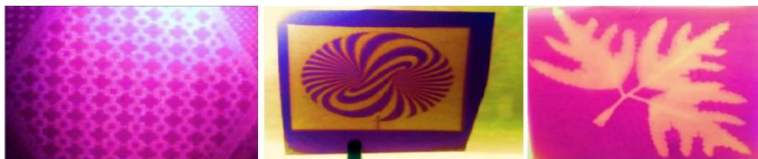
Figure 1. Optical recording images with high contrast by the UV light in SPLC polymer films.
